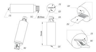
(1) MicroSD card socket, push-push type (2) Bicolor 3-mm device LED (green and red) (3) SeaTalk NG connector of YDVR-03R model (4) NMEA 2000 connector of YDVR-03N model (5) MicroSD card, pin side (6) MicroSD card, label side (7) MicroSD card, plugged in
